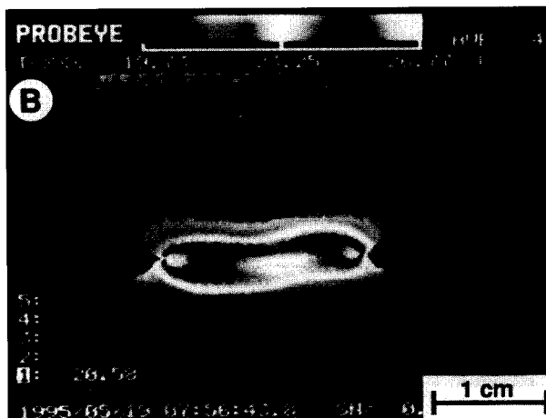
Figure 5 F-x curve of a DDEN-T specimen of COP with l = 20 \text{ mm} and t = 6.05 \text{ mm} (a), along with the serial IT frames taken during loading (b). Note: taking position of the IT frames is indicated in the F-x curve in (a)
