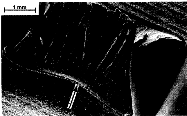
Figure 10 Deformation of the notch plane (arrow indicates) in COP of t \approx 6 mm at a ligament laying below the lower threshold value ( l \approx 4 mm)
